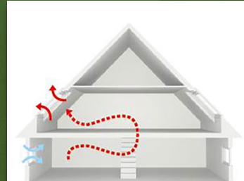
Natural ventilation: Stack effect with open windows
