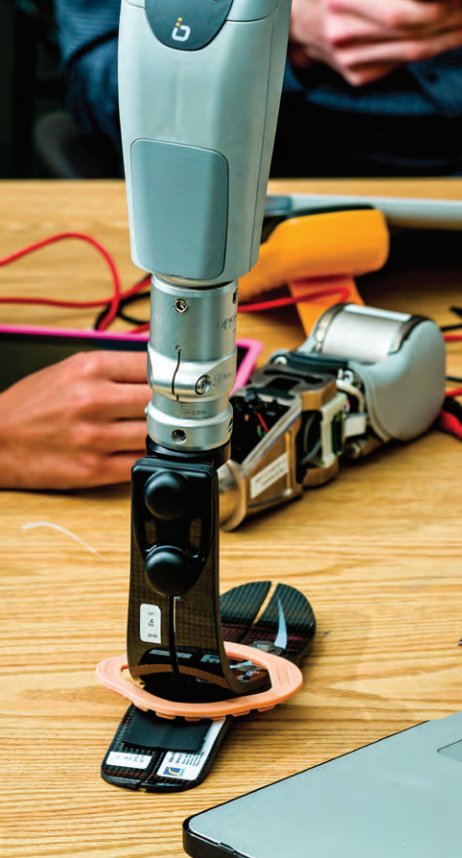
Prosthetics limbs, switches, sensors, and wires are not the typical tools of musicians, but at the University's F.O.R.E. Center they take their rightful place next to pianos and computers—all working together to bring advanced human functionality. Below, Colby Leider discusses engineering intricacies of Össur's Rheo Knee with undergraduate music engineering students who are assisting with the research study.
